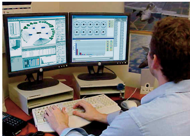
1 VIAssist provides one view for in-depth event analysis (on the left monitor), and a dashboard view of global activity (on the right).
